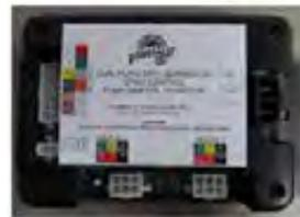
**Fig.1 Slideout Controller**
