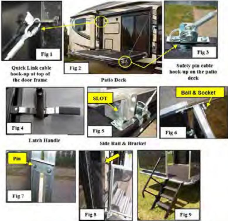
To set up the patio deck, unlatch the two keyed handles from the side of the RV (**Fig 4**). Lower the patio deck until the cables on each side support it. Support cables are attached at the top of the door opening with a quick link (**Fig 1**) and to the deck with a safety pin (**Fig 3**). Patio deck is designed to be folded up with the support cables attached.
