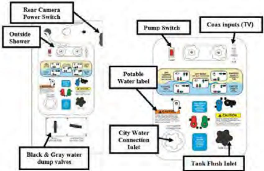
The **Uni-Dock Utility Center** is located in an exterior compartment and allows you to perform the following functions:
