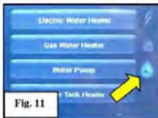
If the pump is shut off from the touchscreens, remote, or Wi-Fi app, the pump will turn OFF, along with the indicator on these devices, but the red switch at the command center stays lit even though the pump is now OFF (also applies to the pump switch at the utility center and the gas/electric water heater). The red switch must be turned off manually for the light to go out.
