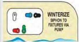
9. Turn the water pump ON with the pump switch on the utility center panel. Antifreeze will be drawn into the water lines when a fixture in the RV is opened. Running antifreeze through the water lines will winterize the tankless style water heater.
